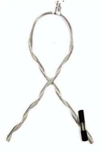
The neoprene component surrounds the bare conductor with a resilient cushioning where the conductor would come into contact with the insulator and with the centre section of the tie. In the case of Side Ties being applied over Armor Rods, the tube can be disposed of, as contact with the bare conductor is prevented by the Armor Rod.
