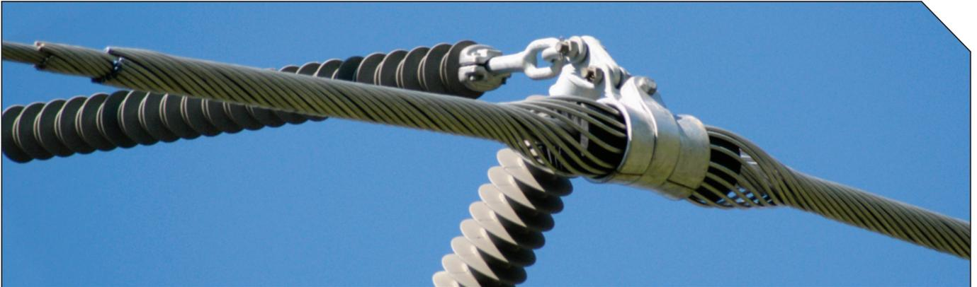
PLP's Thermolign Suspension is specifically designed for application on aluminium based high temperature conductors. The suspension unit is rated for a continuous conductor operating temperature of up to 250°C.
