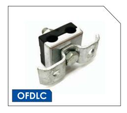
The Fiberlign® Downlead Cushion will accommodate one or two OPGW or other cables as necessary. The base of the clamp is of diecast aluminium, whereas the top is a polymeric material. The base ensures electrical bonding of the OPGW and the top minimises compressive forces which could be transferred through to the optical elements of the cable.
