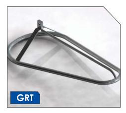
Corona/grading rings are designed to reduce electrical stresses on busbar fittings and overhead and landing span fittings. Manufactured inhouse from extruded aluminium tube, corona rings can be designed to customer requirements. Please contact PLP with required dimensions and specific needs.
