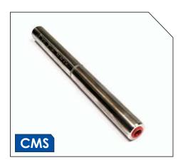
Made from 304 stainless steel, these are single piece fittings for SC/AC and SC/GZ conductors. Designed and manufactured to meet Australian Standards, each fitting is stamped according to conductor stranding size and the recommended compression die A/F size.
