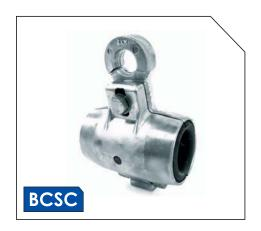
The ASV series of LV ABC Suspension clamps have been developed to protect the integrity of the cable insulation by controlling the cable slip during impact loads. The built-in failure link allows the undamaged cable to drop to the ground, thus providing a coordinated failure mechanism. The clamps are intended for use on straight runs and line deviation angles up to 25°.
