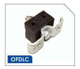
The Fiberlign® Downlead Cushion will accommodate one or two OPGW or ADSS conductors. The base of the clamp is of diecast aluminium, whereas the top is a polymeric material. The base ensures electrical bonding of the OPGW/ADSS and the top minimises compressive forces which could be transferred through to the optical elements of the cable.
