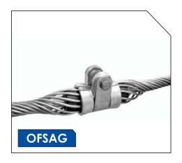
The unit uses the concept of a combination of structural reinforcing rods, outer rods, 'bolted' housing and resilient cable inserts to reduce compression clamping and bending stress on the cable and glass fibers. Effects of wind-induced cable motions such as Aeolian vibration, galloping and wind sway are also minimized.
