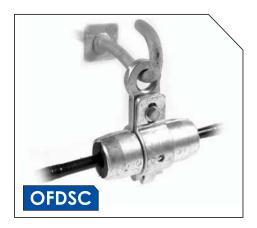
The Fiberlign Dielectric Suspension fitting is intended for use on All-dielectric Self-supporting (ADSS) optical fiber cables, typically installed on distribution power poles. Cushion inserts gently grip the ADSS cable and provide moderate slip strength without damaging the cable jacket.
