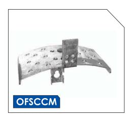
The Fiberlign Cable Storage Bracket is designed to store excess ADSS or underground fibre optic cable. Excess cable can be utilised for future loop joints or T-offs. Two size available to cater for allowable minimum bend radius of fibre optic cable.
