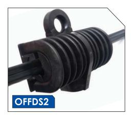
The Fiberlign Dielectric Suspension/Support clamp is a new edition to PLP's ADSS hardware range of products and has been engineered to provide a multipurpose suspension or support clamp for ADSS cable. Cushion inserts gently grip the ADSS cable and provide moderate slip strength without damaging the cable jacket.
