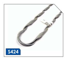
The PREFORMED™ Termination is a strand terminating device which is used by hundreds of electric power utilities, telephone companies, CATV companies and government installations throughout the world. PREFORMED™ Termination provide a superior, as well as economical way to secure guy by using a proven helical concept that provides a constant radial gripping force on the strand.
