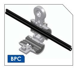
The Fiberlign BPC is design for short urban spans of figure 8 fibre optic cable. The clamp is manufactured from 30% glass filled nylon for superior strength and longevity. Neoprene inserts gently grip the figure 8 cable and provide adequate slip strength without compromising the cable jacket. Installation time is dramatically reduced with the clip/ pin design, requiring next to no tools for installation.
