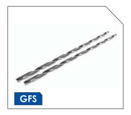
Preformed Strand Splices are used to repair strand or messenger cable simply and economically. Because of its superior design, the Preformed Strand Splice provides maximum strength and excellent fatigue characteristics, resulting in longer life for both strand and messenger.
