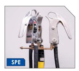
Substation Portable Earths (SPE) are purpose designed to suit a wide range of applications and installation configurations from 5mm up to 120mm in diameter. SPE devices connect between working earth stirrups on busbars and earth stubs or mats.
