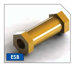
Earthing stubs are made from high purity brass, able to carry fault currents up to 40kA for 0.5 seconds or equivalent and suitable for connection of earthing devices onto structures.
