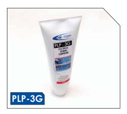
Recommended for all aluminium connections to effectively preserve and protect compression joints. The conductive compound consists of Zinc particles which penetrate oxide films that form on aluminium surfaces. Air and moisture are sealed out, which reduces oxidation and corrosion that would occur on exposed Aluminium. PLP Jointing grease maximises electrical conductivity, while containing thermal properties to endure high temperatures without softening.
