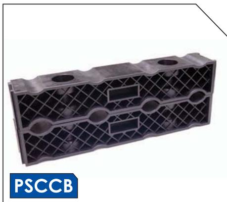
Cable Blocks fasten cable diameters from 12 mm up to 32 mm. By means of 2 block parts, 4 cables can be fastened alongside each other. Additional cables are able to be fastened alongside each other by coupling the block parts together using the standard dovetail connection.
