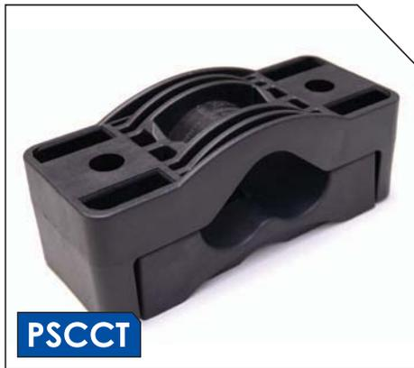
Triple type cable clamps fasten a wide range of single and multi conductor low and high voltage cables in triangular formation. Designed to provide superior mechanical strength, ideal for installations where cables are subject to short circuits. The wide contact area provides a controlled pressure on the cable and prevents damage to the conductor insulation.
