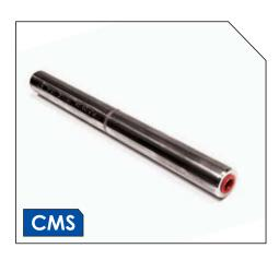
Made from 304 stainless steel, these are single piece fittings for SC/AC and SC/GZ conductors. Designed and manufactured to meet Australian Standards, each fitting is stamped according to conductor stranding size and the recommended compression die A/F size.
